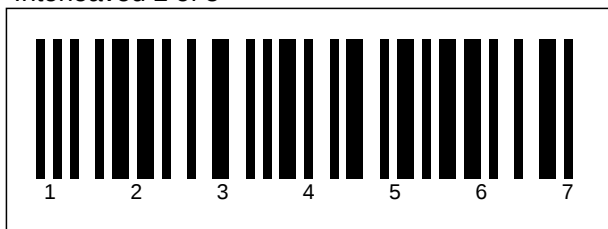
Interleaved 2 of 5 + CHECKSUM
